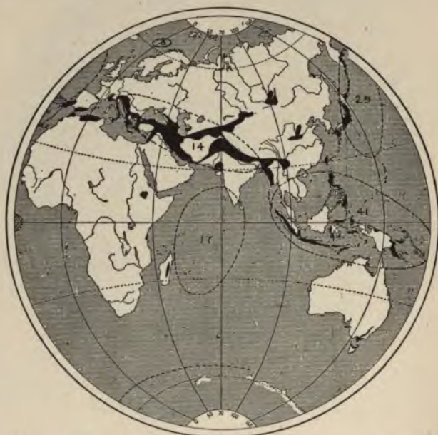
FIG. 16 a.—The earthquake belts and the earthquake "ovals" of the Eastern Hemisphere (after De Montessus and Milne).
